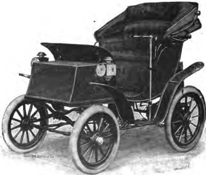
FIG. 447.—Electric Victoria for Carrying Two Passengers. The weight of the carriage shown is about 2,100 pounds; its radius of travel about 40 miles per charge of battery; its maximum speed 13 miles per hour.
